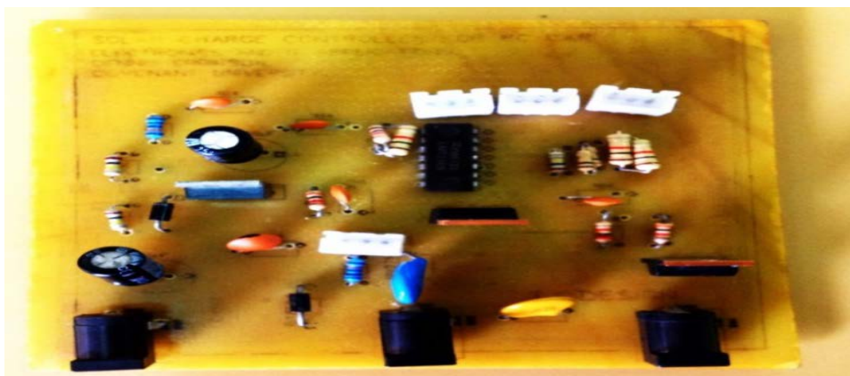
Figure 4: Completed PCB for Solar RC car
